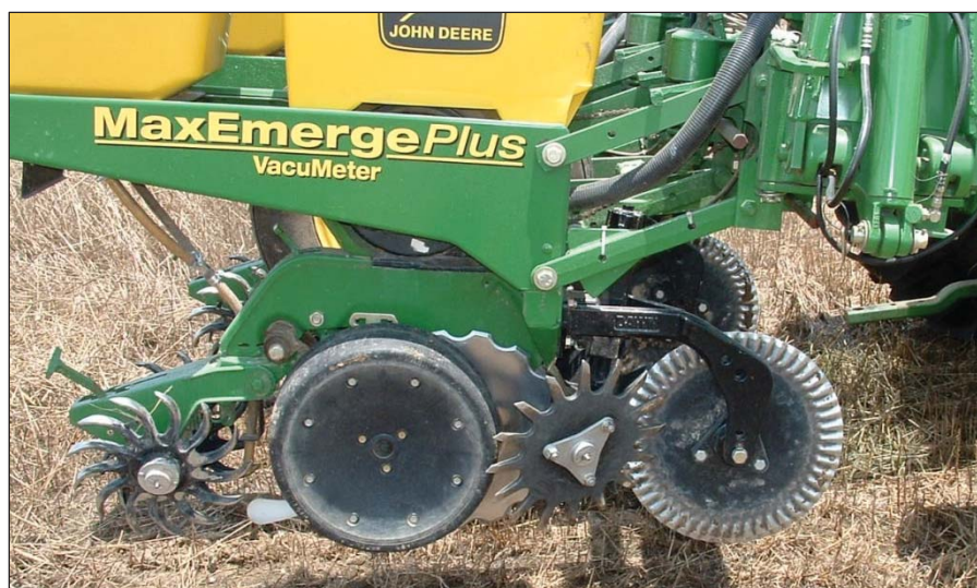
Figure 4. Commercially available DAWN ® row cleaner with fluted coulters and spoked row cleaning wheels behind the coulters.
