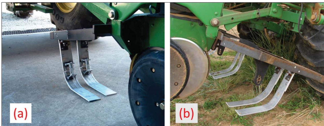
Figure 2. Custom made prototype residue managers: (a) Jointed skis preloaded by sets of springs at the joint line to maintain downward pressure against residue on the soil surface and spaced to accommodate a coulters, (b) Rigid double pressing ski with spacing for a coulters.
